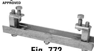
Fig. 772 Adjustable Steel Beam Attachment Size Range: Flange Widths 4" thru 15" Page 11-13
