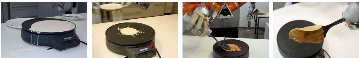
FIGURE 1.6 Physical Behavior Flaws: pancake mixed spilled, spatula placed over the pancake, pancake stuck on spatula. Courtesy: IAS.
