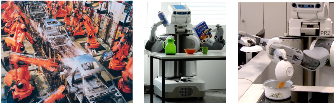
FIGURE 1.2 Robots in an industrial and household setting. Left: Industrial robots perform repetitive tasks with high precision at a car assembly line under real-time conditions. Middle: PR2 performs pick-and-place actions in the context of setting a table for breakfast. Right: PR2 performs a complex meal preparation task in which it pours a granular fluid from a bowl into a preheated cooking pot. Courtesy: ABB (left), IAS (middle, right).
