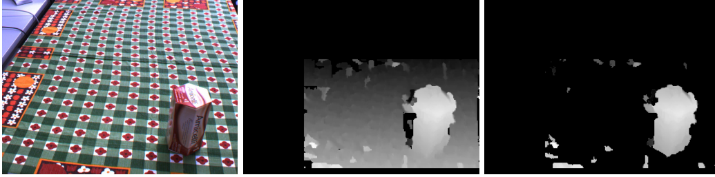
Figure 3.4: Plane subtraction [1]. Left : Original color image. Middle : Disparity image of the color image on its left. Right : Remaining object in the disparity image after the plane subtraction.
