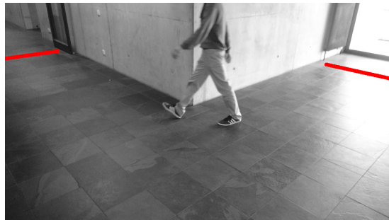
Figure 4.3: Experimental set-up for the parameter calibration of the obstacle utility. Participants were instructed to walk around the corner in both directions. A start and finish line was marked with white masking tape on the floor (here, highlighted in red).
