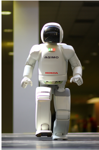
Figure 5.4: An example of a bipedal walking robot. ASIMO can walk, run, walk backwards and climb stairs. (Figure: Wikimedia, Vanillase, 2011 )
