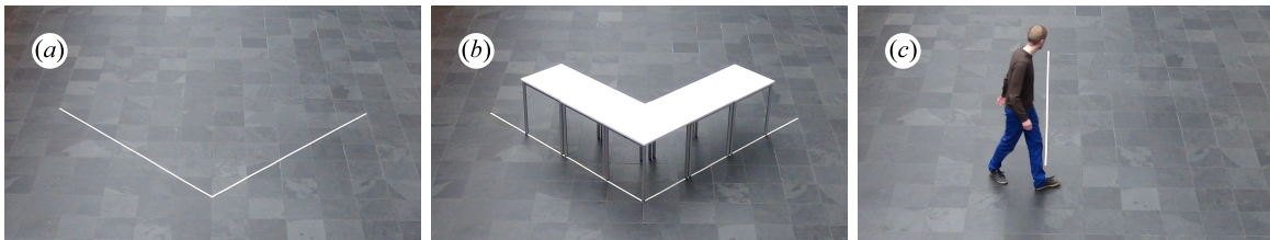
Figure 4.18: Experimental set-up for a series of experiments investigating the change of walking direction. Participants had to walk around the obstacles in both directions. In experiment a, the 90^\circ corner was indicated with white masking tape. In experiment b, the same corner was additionally represented by tables. In experiment c, a straight line was indicated with white masking tape. (Figure: Seitz et al., 2014b)
