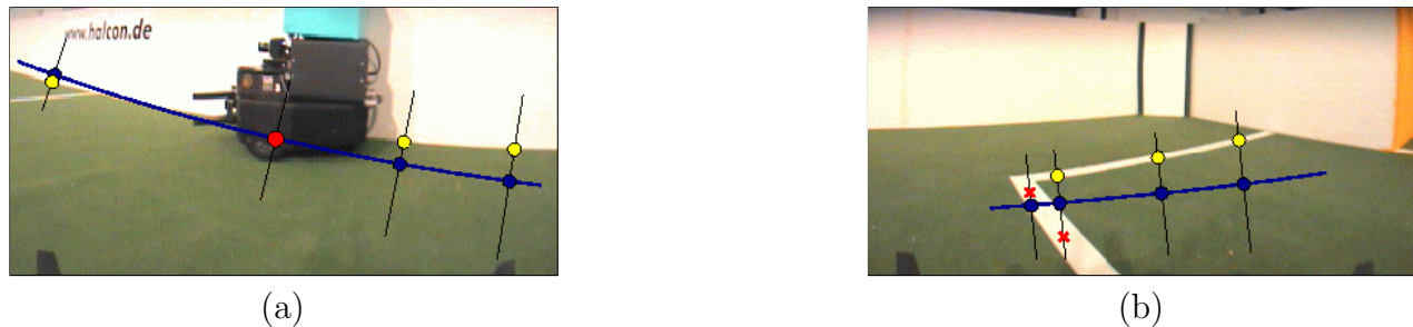
Figure 5.5: Search for correspondences. (a) Due to the occlusion caused by the robot, for one projected point no corresponding image point is found with the required colour transition. (b) By comparing the line width in the image with the line width of the projection, wrong correspondences (crosses) can be detected.
