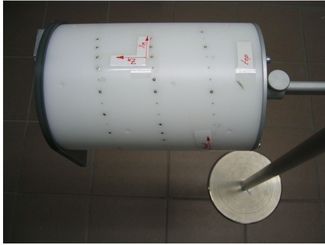
(b) Hollow, cylindrical plastic phantom containing a helical pattern of 54 BBs of two different diameters.
