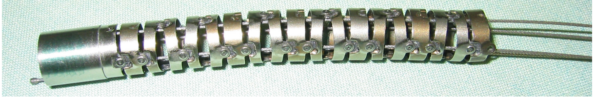
Figure 4.12: Typical bending region usually found in endoscopic instruments. Four cables are pairwise and alternately connected to every second link of the bending region. They are often controlled by steering levers, where two each are connected to the same lever.
