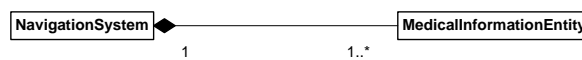
Figure 6.3: The black diamond indicates a composition. The NavigationSystem is composed of MedicalInformationEntities . The number indicates that there is a minimum of one MedicalInformationEntity involved and exactly one NavigationSystem .
