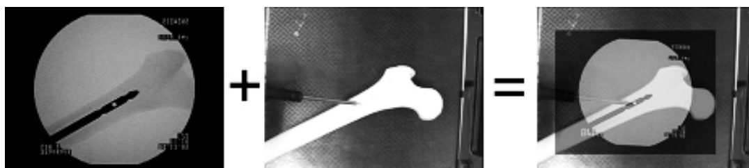
Figure 5.10: The fused video and X-ray image during an intramedullary nail locking of the camera augmented mobile C-arm system provides a guidance interface ideally using only one X-ray image. Images courtesy of Stefan Wiesner and Sandro-Michael Heining.
