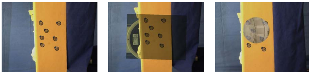
(a) Image of the orthogonally mounted camera. (b) Gantry mounted camera image overlay after applying H_{I_o^0 \leftarrow I_g^{90}} . (c) X-ray image overlay after applying H_{I_o^0 \leftarrow I_x^{90}} .
