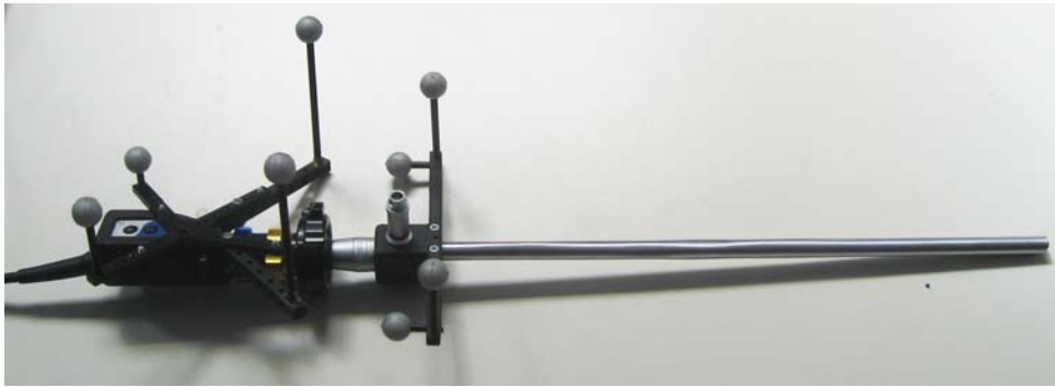
Figure 1.8: A laparoscope with a oblique viewing 30 degree optic. The laparoscope is extended by tracking targets to enable soft tissue navigation as proposed by Feuerstein et al. [55].
