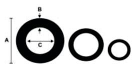
Outside Diameter Tolerance = plus .004" / minus .000" Inside Diameter Tolerance = plus .000" / minus .008"
