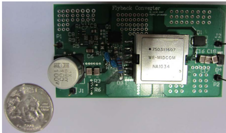
Figure 27 Prototype of PV balancers in Architecture I and Frontend Converter in Architecture II
