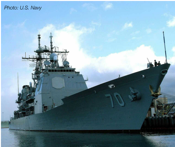
The USS Lake Erie (CG-70) with its SPY-1B radar panel clearly visible
