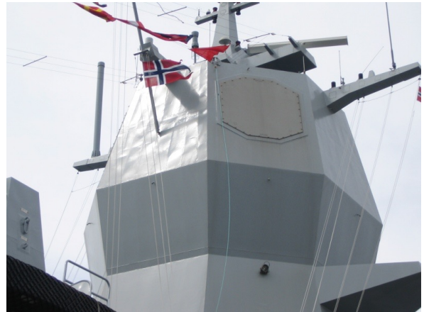
A smaller variant of SPY-1, the SPY-1F radar, atop a Norwegian Fridtjof Nansen-class Aegis frigate
