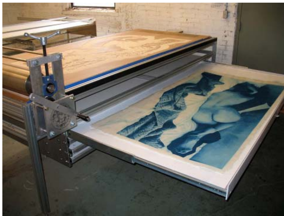
Large woodblock press in operation, August 2006. Paper delivery drawer visible at top left in background. Press with block sucked down onto vacuum plenum, paper take-up drawer open with just completed print. Press itself is just over 5 feet wide by 10 feet long and paper drawers are 4 x 8 feet..
