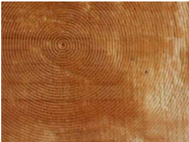
detail showing the carving of the spiral tool path
