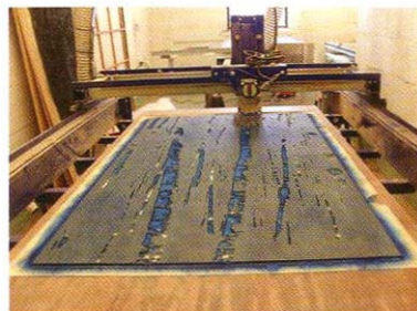
Figure 168. One of 12 woodblocks for Aspen Grove , by Mike Lyon, during carving on a ShopBot CNC router. Aspen Grove is a reduction woodcut – there was only a single block, carved and re-carved in stages, with a printing after each re-carving. In this photo, the carved areas (which are blue) were carved prior to the next printing – new carving is evidenced by lighter areas of the block. Image courtesy of the artist.
