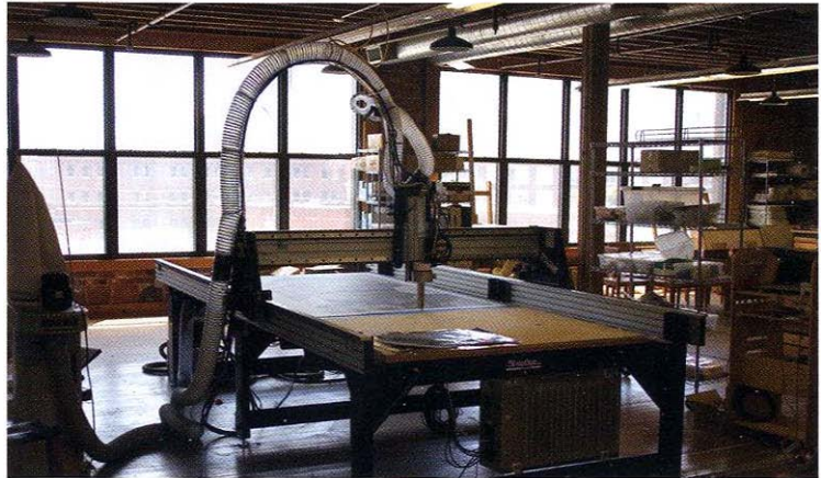
Figure 177. Large ShopBot router at Mike Lyon's studio in Kansas City. The router is set up to hold an ink pen that is raised and lowered via a custom solenoid headstock designed by Lyon. Image courtesy of the artist.
