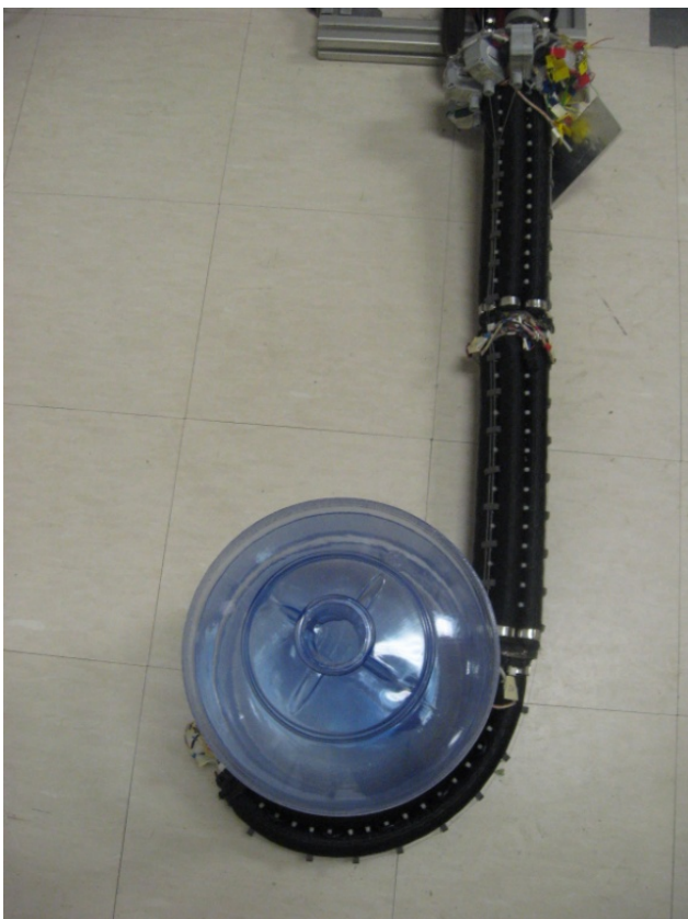
Figure 6b. The same object grasped using the tip section of the Octarm.
