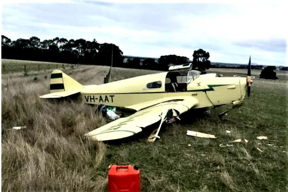
VH-AAT (c/n 193) Michael Stalls, Wangaratta, Victoria, Australia. This was an airworthy surviving Miles Aircraft, that is until it was forced landed at Lilydale on 17.4.20 due to fuel starvation (caused by the owner not cleaning the fuel pipes following a long time in storage, during which the petrol had jellified). The photograph below shows the extensive damage to the port wing and undercarriage following the forced landing.
