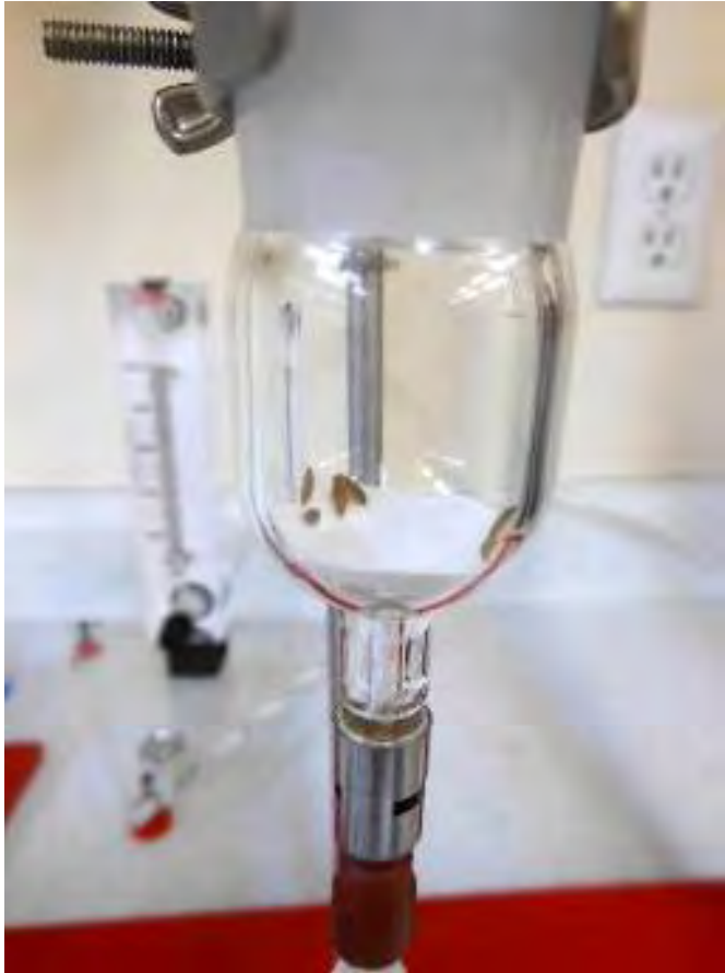
Fig. 3: Multiple adult virgin female Thylocryptus contractus placed together to collect potential sex pheromone in the head space above with the Porapak Q column.
