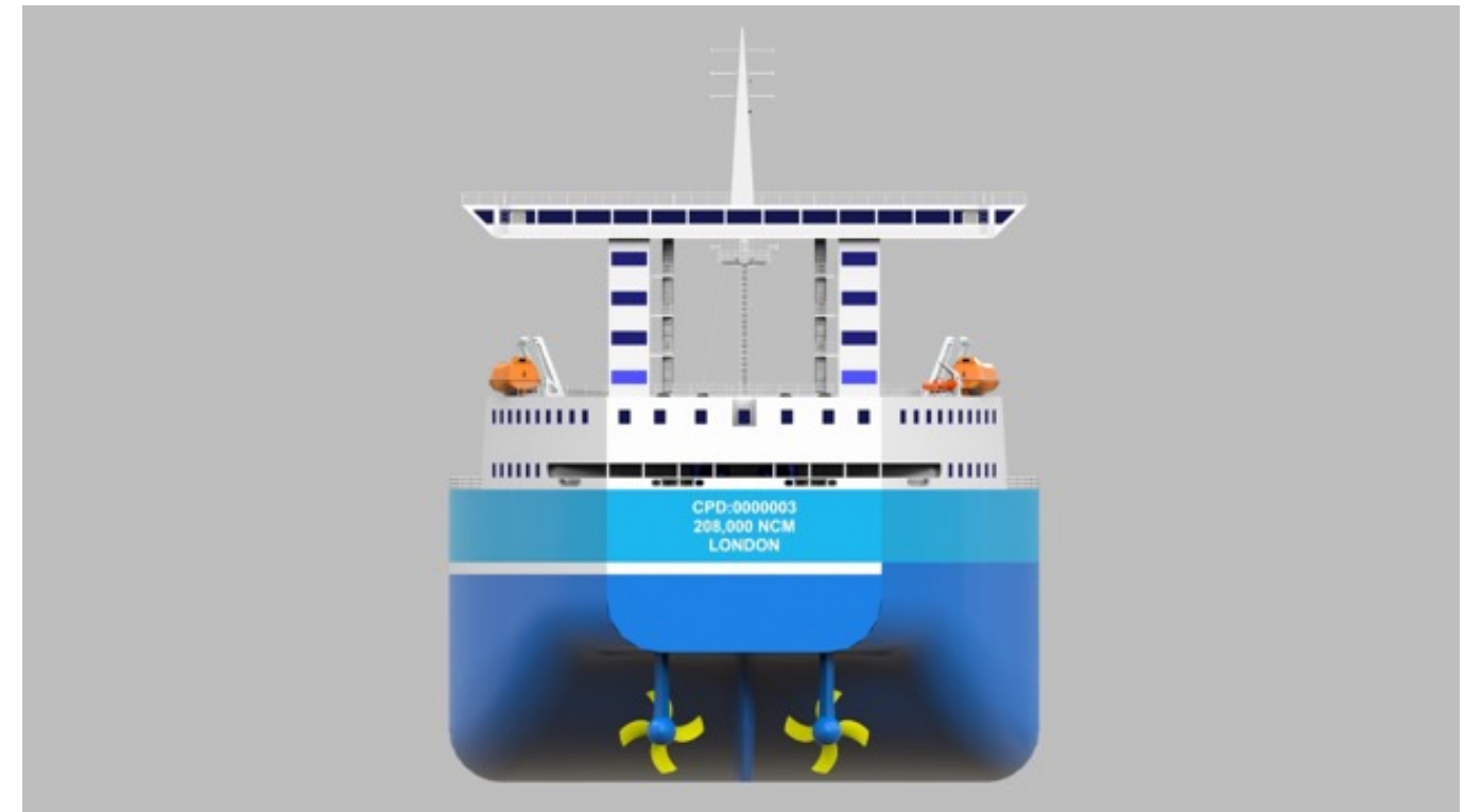
Figure 38: Concept design of a nuclear-electric Capesize bulk carrier – Courtesy CORE POWER.
