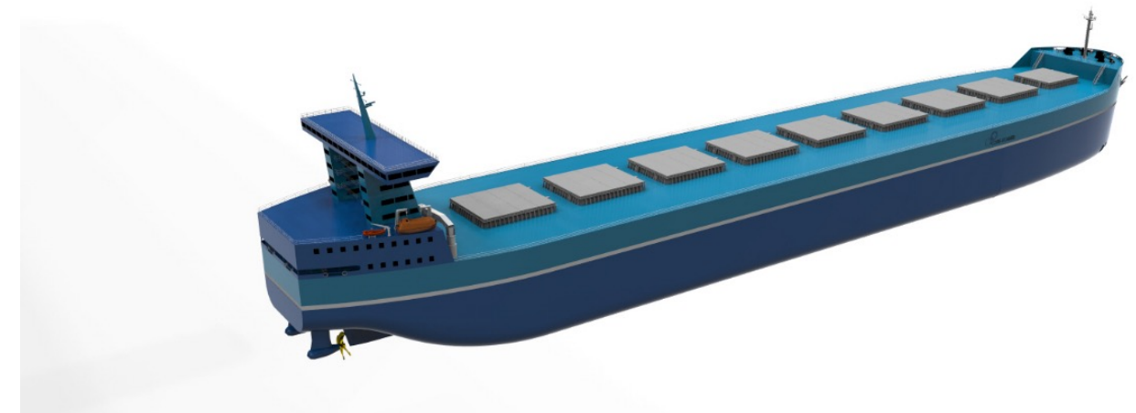
Figure 33: Concept design of a large bulk carrier powered by a molten salt reactor – Courtesy CORE POWER
