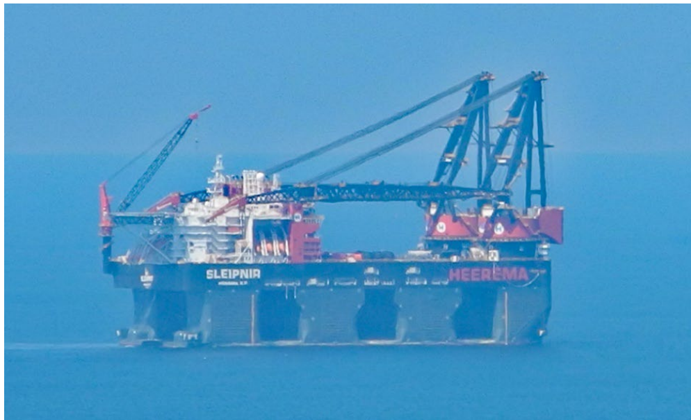
Figure 9. SSCV (Semi-submersible crane vessel) Sleipnir: weighing over 300,000 short tons with 96 MW of installed power on board. From: Wikimedia Commons.
