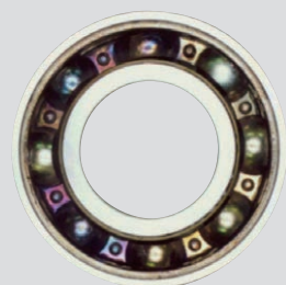
Grease packed bearings (failure due to grease leakage)
