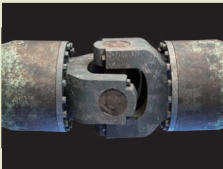
Photo showing condition of U-joint after operation
