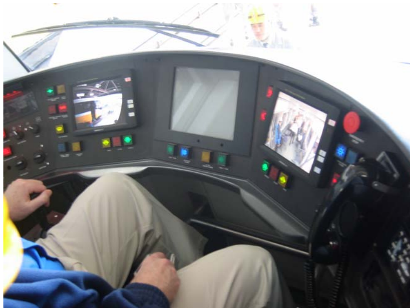
FIGURE 13 Ergonomic cab with video monitoring.
