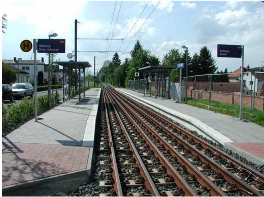
Track sharing: different width of vehicles: 2,40; 2,65; 3,00 m. 10
