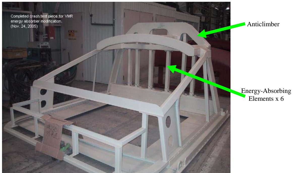
FIGURE 5 Controlled collapse cab structure prior to crush test.
