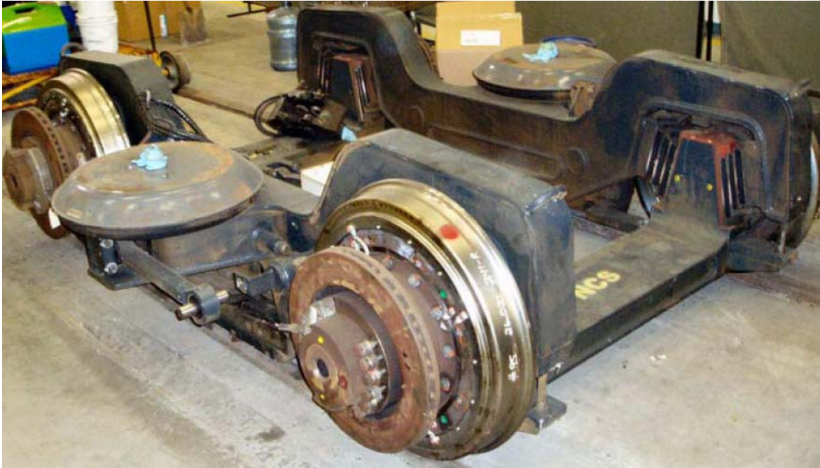
FIGURE 5 Center truck, Kinki-Sharyo LFLRV, Newark Subway.
