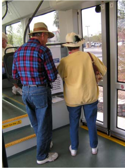
FIGURE 11 Fully glazed doors.
