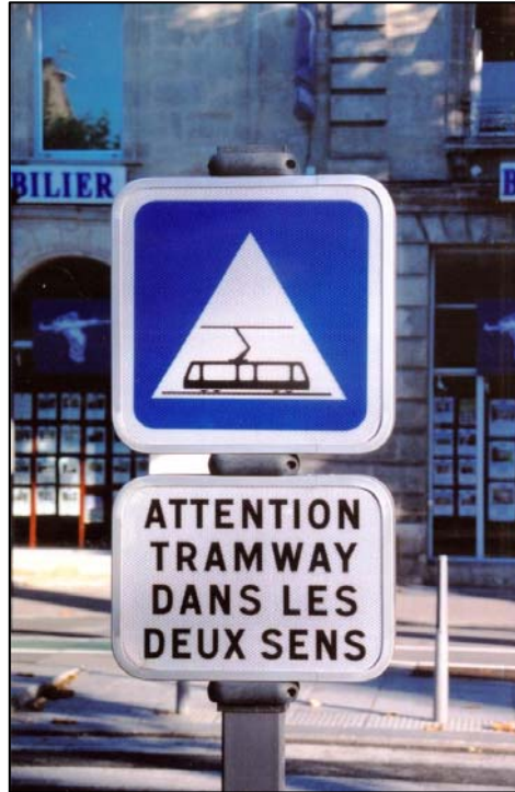
FIGURE 7 Two-way LRV warning sign with LRV symbol, Bordeaux, France (urban environment, median operation).
