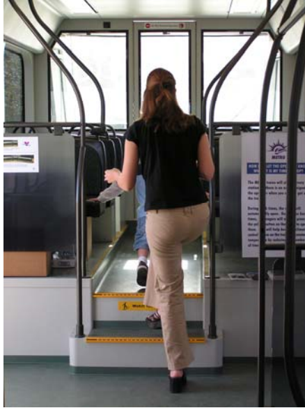
FIGURE 8 Transition from low- to high-floor area.
