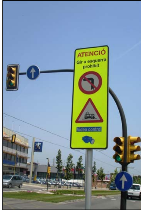
FIGURE 16 Video enforcement of left-turn prohibitions (regulatory and warning sign combination), Barcelona, Spain (urban environment, median operation).
