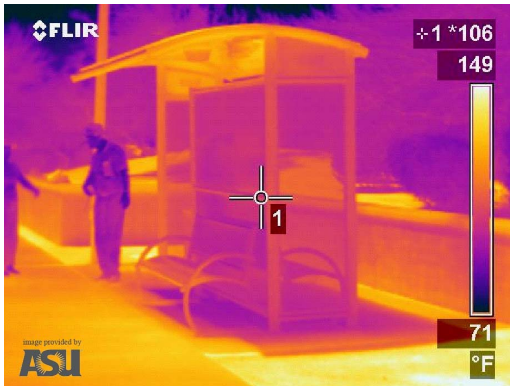
FIGURE 8 Radiant image of passenger waiting shelter.
