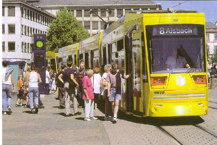
FIGURE 5 Darmstadt: street-level boarding of low-floor tram.
