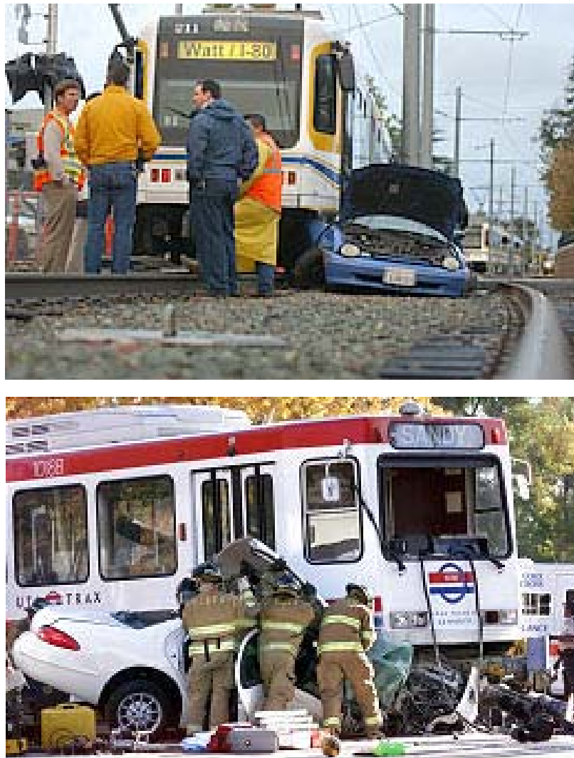
FIGURE 3 Override collision behaviors between LRVs and automobiles (13, 14).
