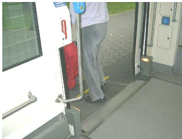
FIGURE 4 Retractable ADA-compliant ramp on Portland streetcar. (Photo by Lyndon Henry.)
