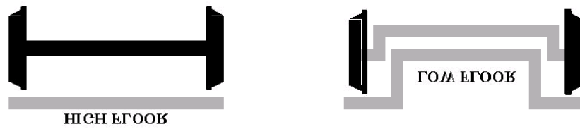
FIGURE 1 Independent rotating wheels on a nonrotating cranked axle.
