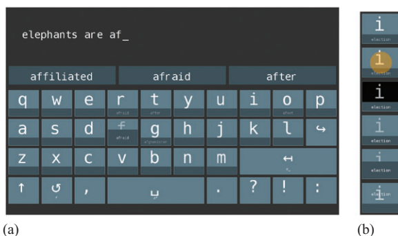
Figure 5.3 Eye typing interface of GazeTheKey [32]: (a) suggestions are embedded to keys and (b) multi-step dwell time is used for selections of firstly the letter and secondly the suggestion
