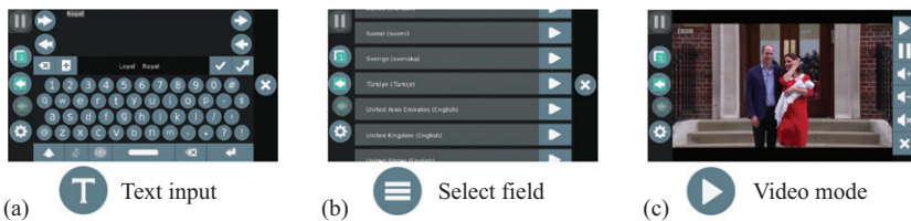
Figure 5.13 Gaze-sensitive icons on a webpage are associated with gaze-controlled interface modes for sophisticated gaze-based interaction: (a) virtual keyboard for text input, (b) list of options from select field, and (c) mode with video controls
