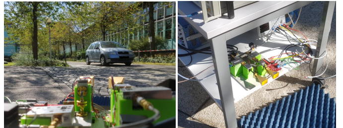
Fig. 13. Measurement scene comprising a moving vehicle from sensor point of view (left) and the top view of sensor (right).
