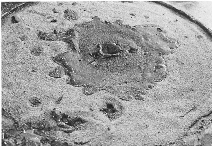
Fig. 11.6. Shot 800426. The target consisted of viscous clay overlain with \sim 20 mm of ice and an upper regolith layer a few mm thick of sand-sized shell particles. An impact of a 6.4-mm pyrex projectile at 1.76 \text{ km s}^{-1} fractured the ice and produced a flat-floored crater. A central secondary crater resulted from fallback of a blob of clay ejecta held together by surface tension.
