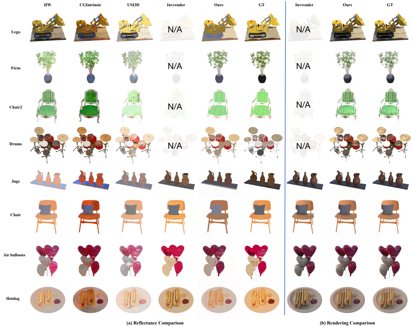
Figure B2: Qualitative Comparison Results of Reflectance and Rendering with Previous Work on the Blender Object Dataset. The top 4 rows represent the sample of our dataset and the bottom 4 rows represent the sample of the Invreder dataset. Our method can perform reflectance estimation and novel view synthesis on both datasets well, while Invreder [7] fails to do that on our dataset. N/A means failure.
