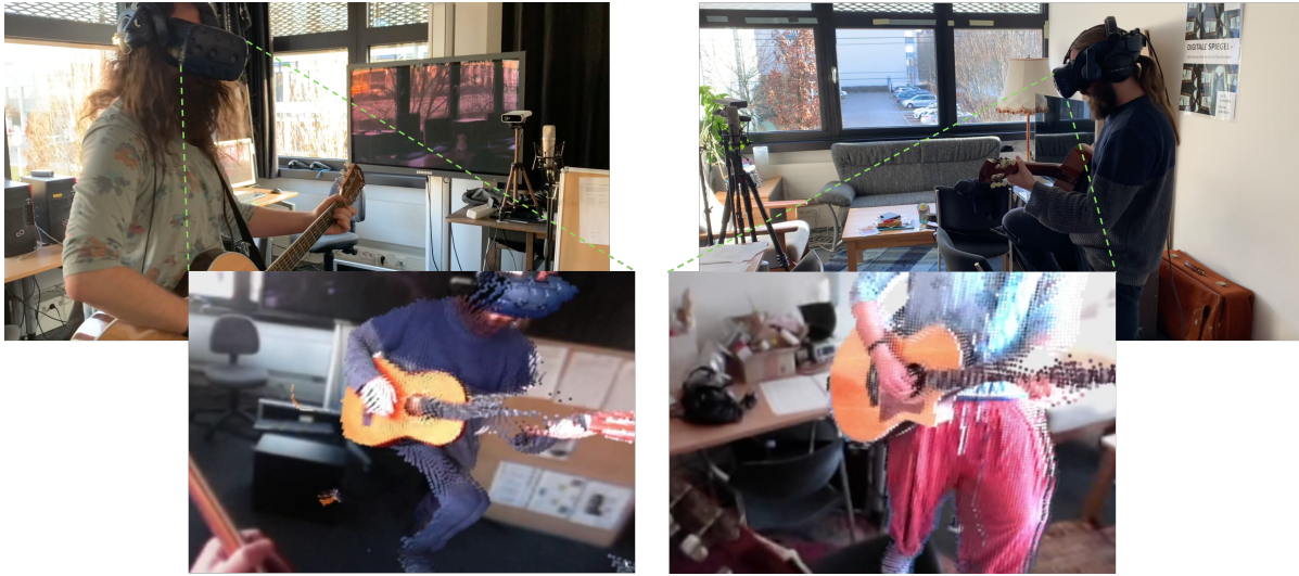
Figure 1: Two jamming partners in separate rooms and their mixed reality views featuring 3D point clouds during a jam session.
