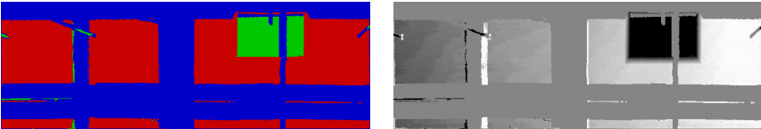
Fig. 8.5: Left: Labels (red occupied, blue occluded, green empty). Right: Corresponding depth image.
