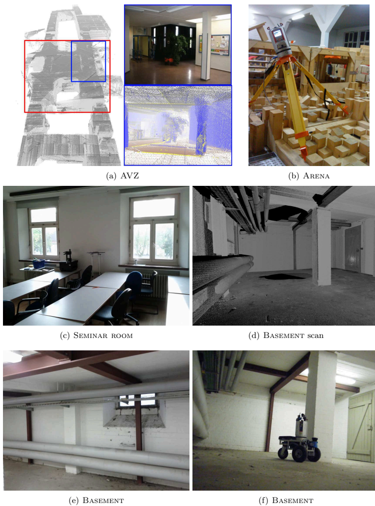
Fig. 3.11: (a) The complete 3D map of AVZ as seen from above. The red box marks the area used for the experiments in Section 4.3.4. The blue box marks the area shown on the right. (b) The Riegl-VZ on a tripod during data acquisition in the ARENA. (c) Photo of the SEMINAR ROOM and (e)+(f) BASEMENT environment. (d) A scan showing approximately the same area as (f).
