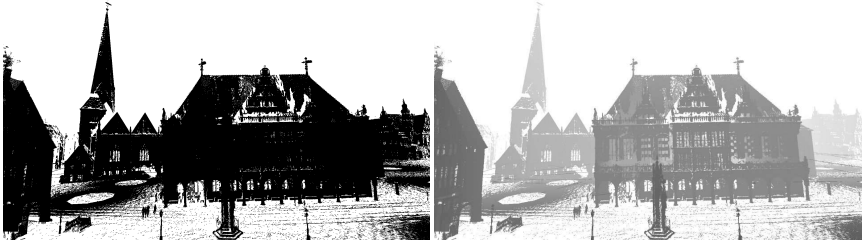
Fig. 4.5: The effect of fog onto the depth perception on one scan from the BREMEN CITY data set. Left: The points cloud without fog. Right: Exponential white fog with a density of D = 0.015 m.
