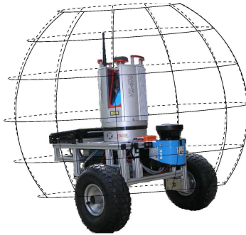
Fig. 4.9: The scanned environment corresponds to a partial sphere, restricted by the field of view of the scanner. The scanner is located in the center.
