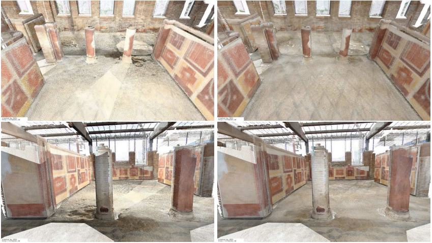
Fig. 8.33: OSTIA ANTICA. Details from the point cloud before (left) and after optimization (right). Over- and underexposed images are aligned radiometrically thus increasing the homogeneity in the brightness distribution. The point density is identical for all images.
