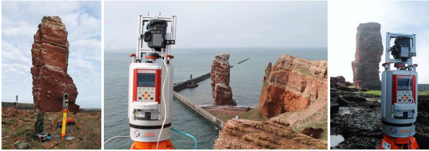
Fig. 3.8: The scanner setup in three selected positions. The Scanner was carried with the backpack seen in the left image and mounted on the tripod.
