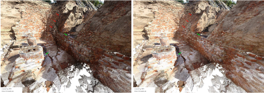
Fig. 8.32: Stephanitorzinger, Bremen, Germany. Details from the point cloud before (left) and after optimization (right) with equal point density. Note the scattered dark pattern on the brick wall, which disappeared after exposure correction.
