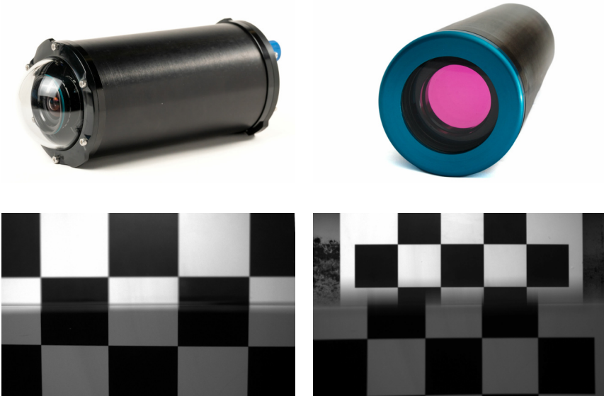
Fig. 3.3: Dome port (top left) and flat port (top right) underwater camera. Below are two example images with the dome port (bottom left) and flat port (bottom right) partially submerged in water. The top half of the image is in air, while the bottom half is in water.
