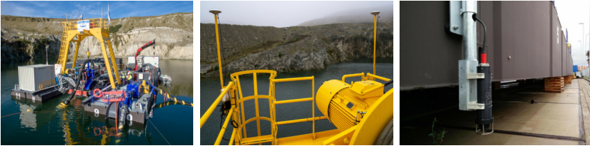
Fig. 7.4: Left: Launch and recovery vessel (Source: ¡VAMOS! project [318]). Middle: GNSS antennas mounted on top of the portal crane tower. Right: SBL transceivers mounted on the corners of the vessel (Source: [214]).
