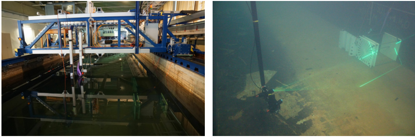
Fig. 6.6: Mobile data acquisition experiments conducted in the towing tank of the chair of fluid dynamics at the University of Rostock. Left: Towing tank at the chair of fluid dynamics in Rostock, Right: Underwater laser scanner deployed in the tank.
