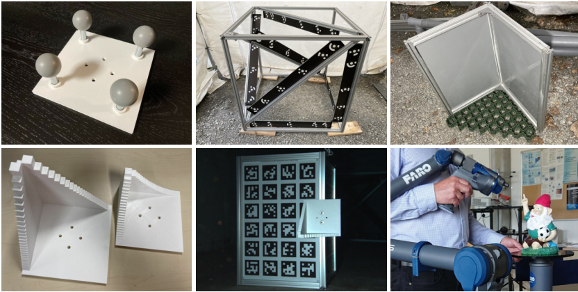
Fig. 4.23: Reference artifacts. From top left to bottom right: Sphere target, Scalebars in a 1\text{ m}^3 measurement volume, Grey painted float glass planes, resolution test targets, resolution test target mounted to calibration fixture, dwarf figure being scanned with the FARO ScanArm.
