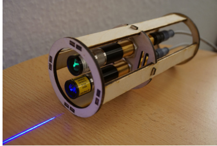
Fig. 5.7: Cross line laser projector in wooden frame employed for the experiments.
