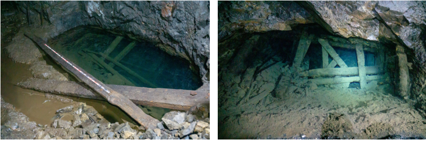
Fig. 1.5: Flooded mine shafts with historic timber installations.
