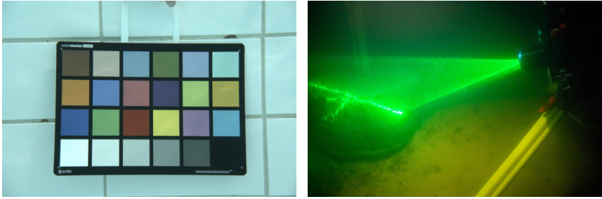
Fig. 2.1: Examples of underwater images. Left: Blue-green color cast visible in an uncorrected underwater image of a color checker photographed at a distance of approximately 1 m. Right: Scattered light of a green laser projector due to particles in the water.
