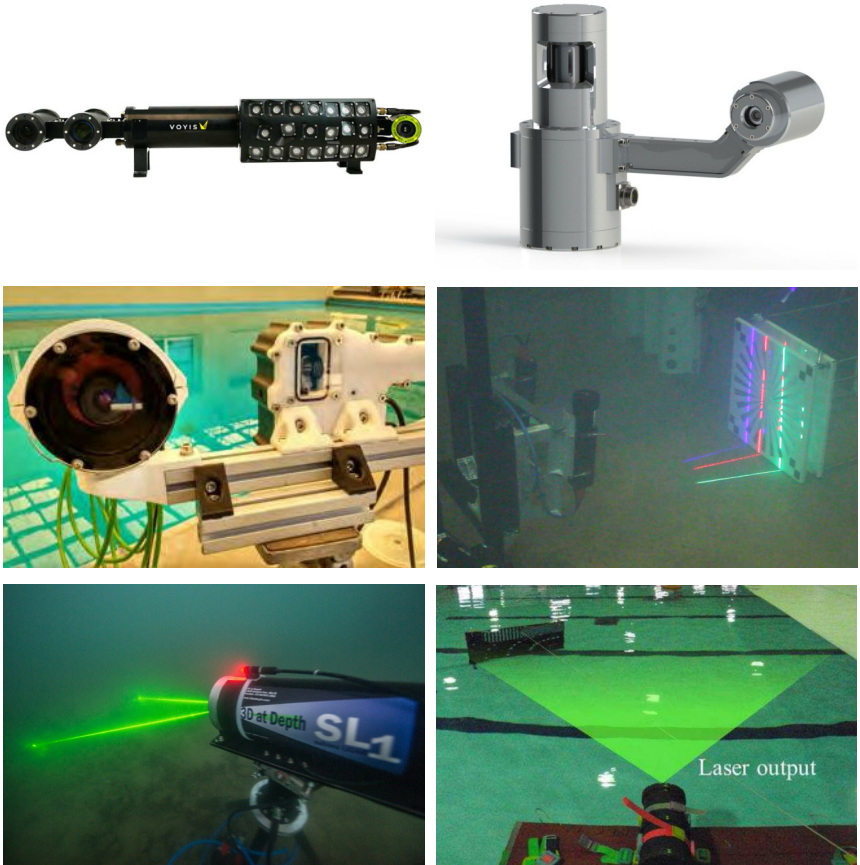
Fig. 2.12: Examples of different underwater laser line scanning systems and Time-of-Flight (ToF) laser scanners. Top left: Voyis Insight Micro / 2G Robotics ULS-500 Micro (Source: [329]). Top right: Newton Labs M4000UW underwater laser scanner (Source: [240]). Middle left: University of Girona underwater laser scanner with galvanometer projector (Source: [256]). Middle right: Kraken Robotics SeaVision Subsea 3D Laser imaging system with tri-color lasers [109, 186]. Bottom left: 3D at Depth SL1 subsea Light Detection and Ranging (LIDAR) (Source: [150]). Bottom right: Mitsubishi underwater laser scanner U4LE (Source: [163]).
