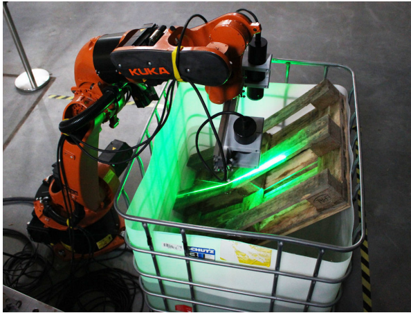
Fig. 4.39: Prototype underwater line laser scanner mounted on an industrial manipulator for scanning a semi-submerged scene.
