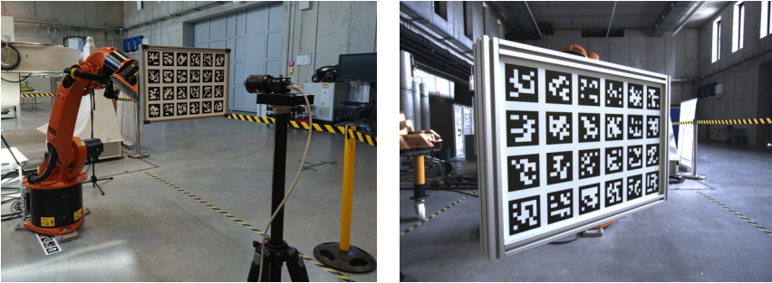
Fig. 3.13: Dataset of Leutert [195] for the evaluation of camera calibration. Left: Experimental setup using KUKA industrial manipulator (Source: [195]). Right: Example image of the dataset (Source: [195]).
