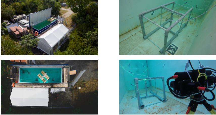
Fig. 4.18: Scanning setup in the test tank. Left: 40 m 3 roll-off container. Right: Underwater scanning of a test structure constructed from aluminum profiles and polypropylene pipes.
