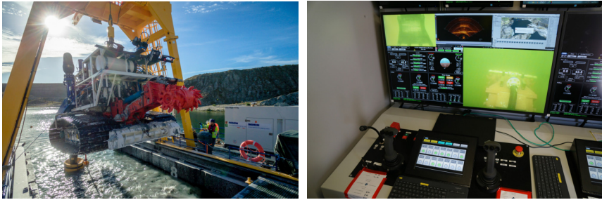
Fig. 7.1: Left: iVAMOS! mining vehicle hoisted on the crane of the launch and recovery vessel (Source: iVAMOS! project [318]). Right: Camera feeds of the mining vehicle displayed in the control cabin.
