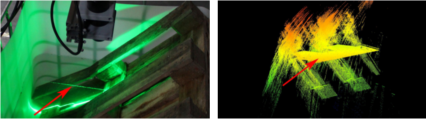
Fig. 4.40: Reflections of the laser line projector on the water surface are exploited to estimate the water plane. Left: Reflection of laser line. Right: Reconstructed point cloud including the water plane.
