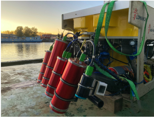
Fig. 6.11: UWSensor mounted in the manipulator of a light Work-Class ROV.
