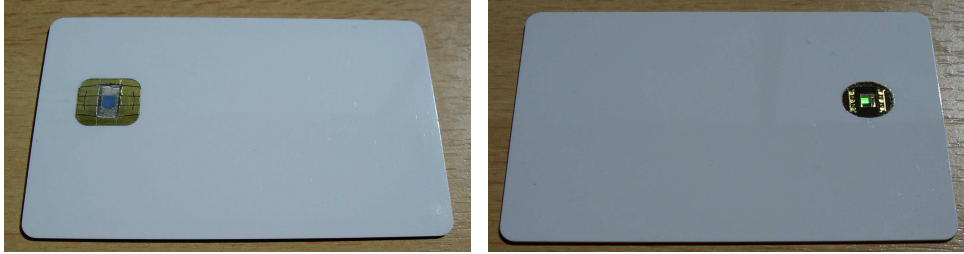
Figure 1.3: Smart card depackaging on the back side (on the right) and on the front side (on the left).
