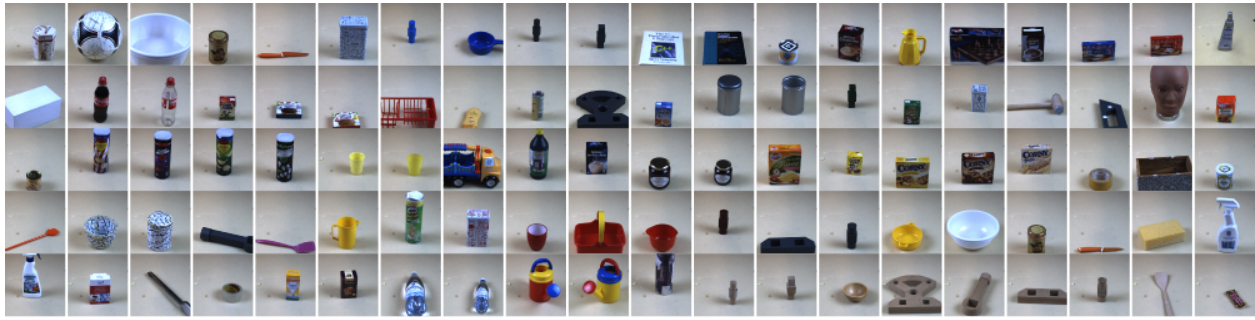
Fig. 8. Multi-view dataset of 100 objects shown in thumbnails. The set contains RGBD and stereo images: 30 samples each object from three camera views. The data were captured under three lighting conditions. The dataset is available at http://caro.sdu.dk/sdu-dataset .
