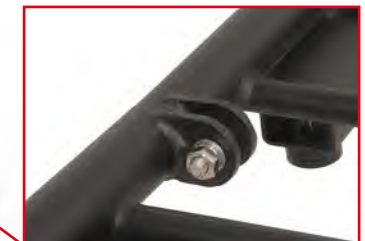
HEAVY DUTY 2" 0.120 WALL TUBING
