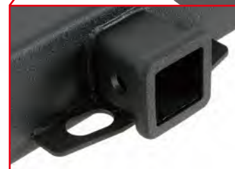
CLASS III RATED 2" RECEIVER HITCH
