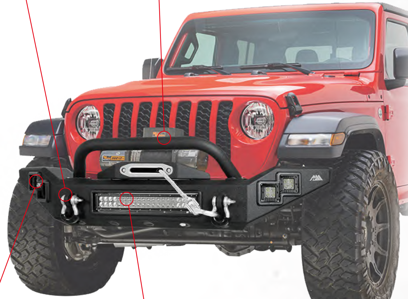
D-RING MOUNTS WELDED INSIDE AND OUT
