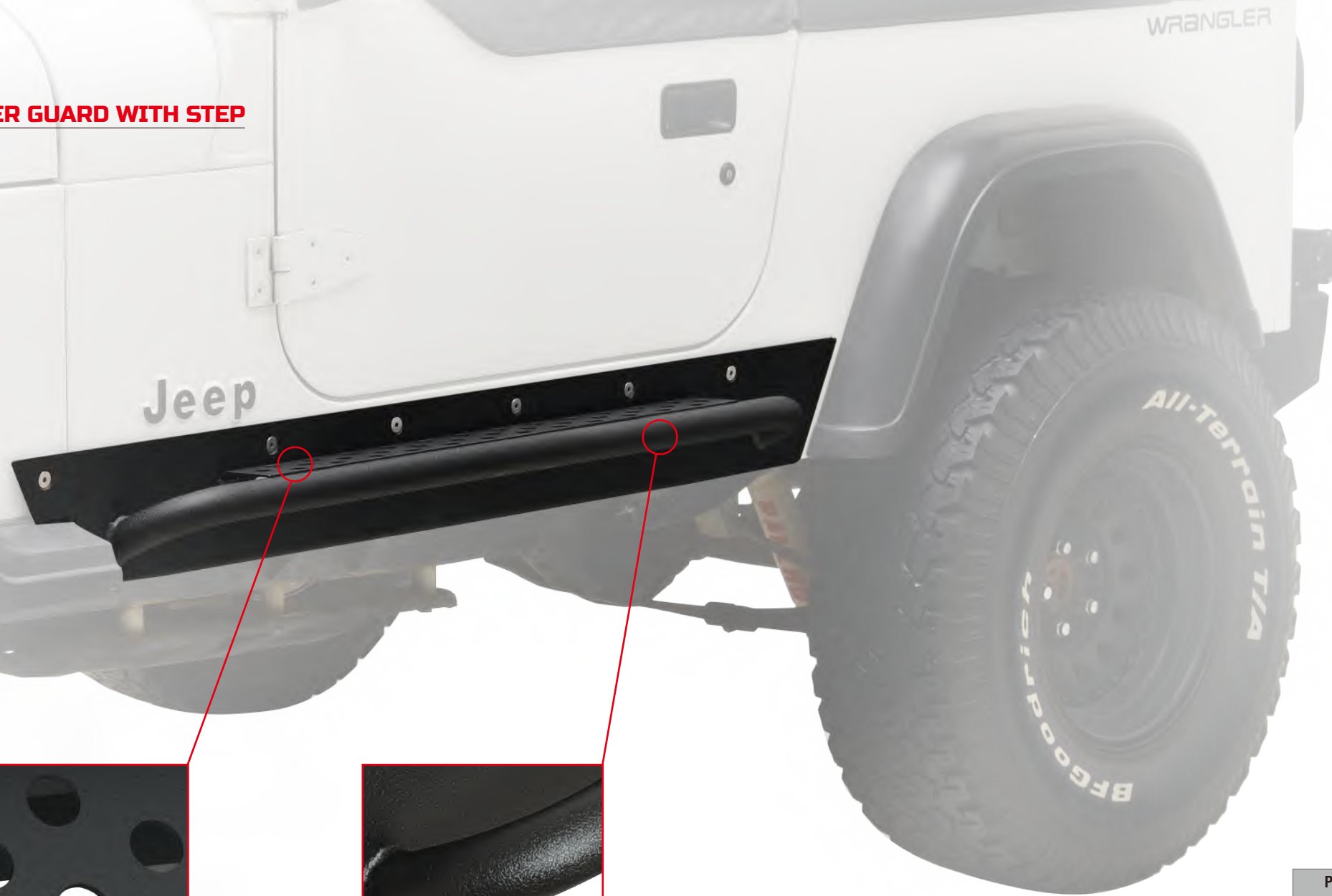
DURABLE 4MM STEEL SHEET
