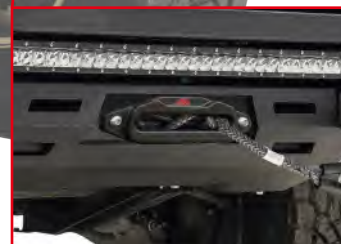
RECESSED WINCH MOUNT WITH INTEGRATED FAIRLEAD PLATE
