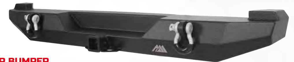
D-RING MOUNTS WELDED INSIDE AND OUT
