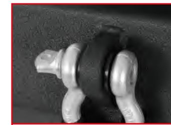
D-RING MOUNTS WELDED INSIDE AND OUT
