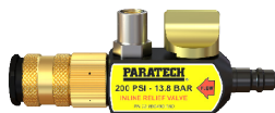
INLINE RELIEF VALVE FOR G3 165 psi / 11,4 bar Designed to relieve over-pressurization and allow a lift bag to remain inflated under a load. This valve will relieve excess pressure from an inflated bag caused by load shifts or temperature changes. Net Weight: 1.0lb 0,4kg Part No. 22-890490-180
