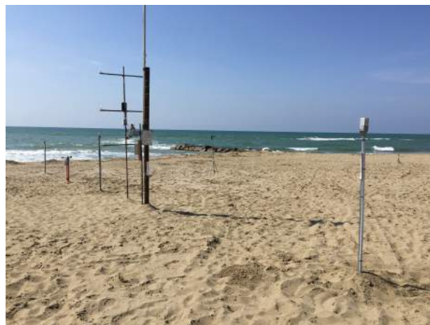
Figure 4. A deployed Beach Wireless Sensor Network (WSN).
