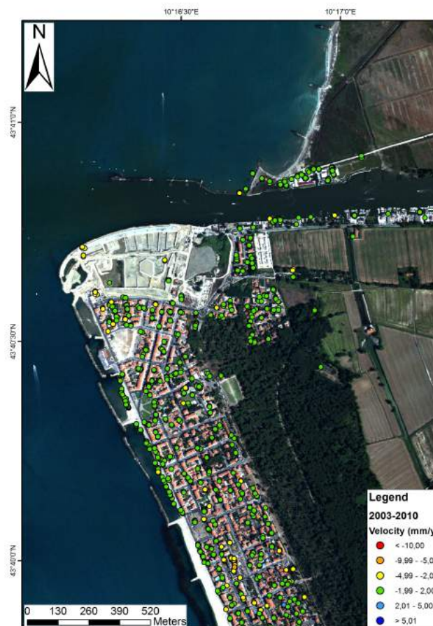
Figure 1. Ground deformation velocity map obtained using Envisat Synthetic Aperture Radar (SAR) data (period 2003–2010) on a true color image in RGB mode (8,5,2) of the study area acquired using the airborne multispectral sensor Daedalus.
