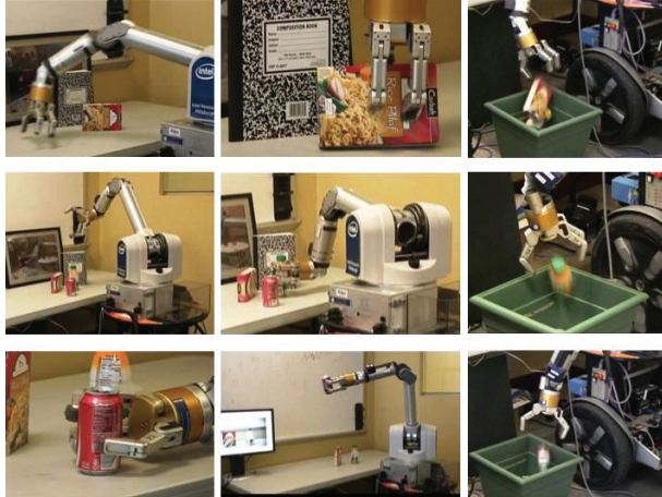
Fig. 9. Snapshots from three runs of three trajectories planned using CBiRRT2. Top row: Grasping and throwing away a box of rice. Middle row: Grasping and throwing away a juice bottle. Bottom row: Grasping and throwing away a soda can.
