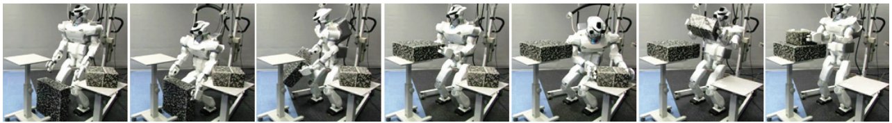
Fig. 14. Snapshots from the execution of the box stacking task on the HRP3 robot.
