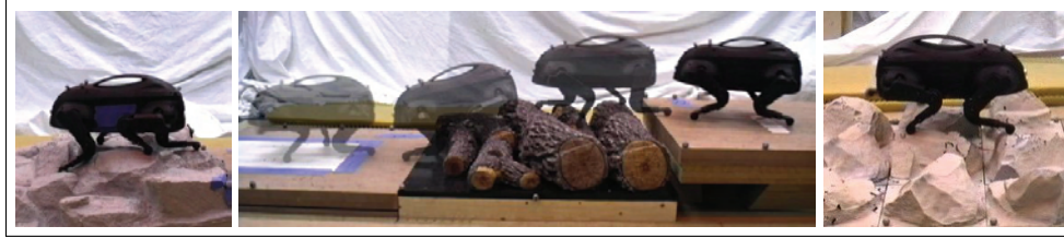
Fig. 25. Boston Dynamics Inc. LittleDog quadruped robot, shown crossing several types of rough terrain. (Images reproduced with permission from Zucker et al. (2011).)
