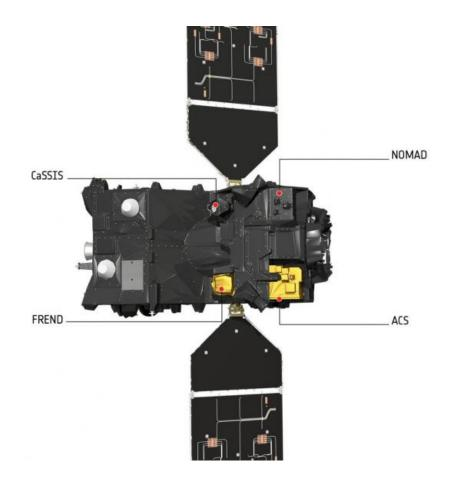
Artist's impression of the ExoMars 2016 Trace Gas Orbiter (TGO) with its instrument packages labelled. Credit: ESA/ATG medialab
