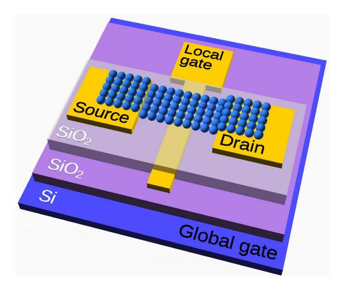
New transistor concept. Thin films made of metal nanoparticles (blue spheres) are electrically contacted by gold electrodes (source/drain). The current flowing through the films is adjustable by the voltage of a local electrode located below the film (local gate). Credit: Christian Klinke, University of Hamburg
