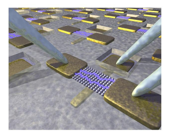
New transistor concept. Thin films made of metal nanoparticles (gray spheres) are electrically contacted by gold electrodes. The current flowing through the films (in blue) is adjustable by the voltage of a local electrode located below the film. For the characterization, needle-shaped probes are applied to the electrodes which provide the corresponding voltages and measure the current. Credit: Christian Klinke, University of Hamburg
