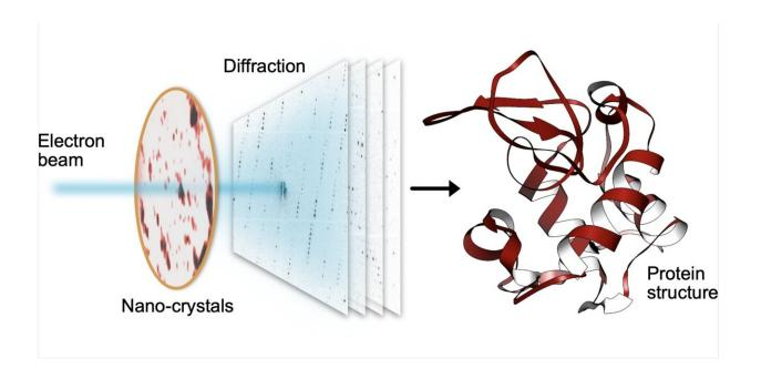
In serial electron diffraction, a small electron beam sequentially hits thousands of tiny crystals made from proteins, which scatter the beam into diffraction patterns. From those patterns, the structure of the proteins can be determined with high resolution. Credit: Robert Bücker
