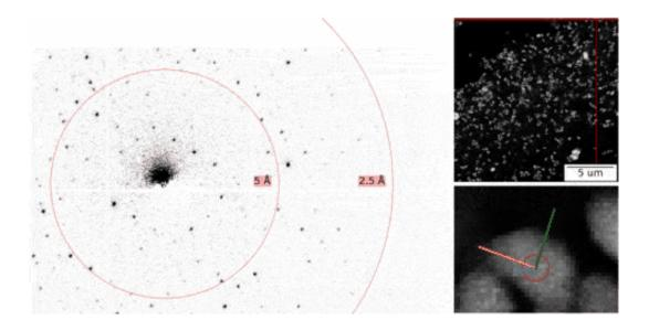
A slow-motion movie of collecting diffraction patterns (left) from thousands of tiny crystals (right) in an electron microscope. Credit: Robert Bücker
