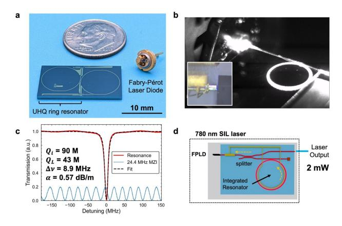
Hybrid-integrated chip-scale 780 nm self-injection locked laser. Credit: *Scientific Reports* (2024). DOI: 10.1038/s41598-024-76699-x
