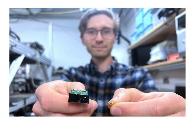
Andrei Isichenko holds the ultra-high-quality ring resonator (left), which can help turn the "coarse" light from a commercially available Fabry-Perot laser diode (right) into a low linewidth laser. Credit: Sonia Fernandez, UC Santa Barbara
