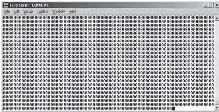
Figure 8.12: Notice I “paced” the transmission in Code Snippet 8.4. After the first A was sent, each A thereafter was sent one per second ( delay_ms(1000) ).
