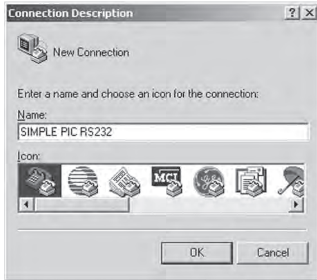
Figure 8.7: Doing this allows you to save the HyperTerminal session with a name for later use.
