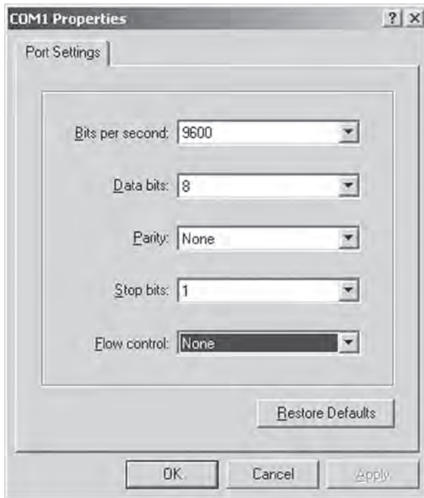
Figure 8.9: No modem control or software signals (flow control) are needed in a simple three-wire RS-232 connection.
