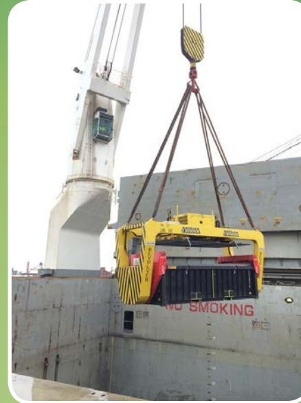
Patented lid lifter in use.
