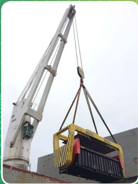
Patented lid lifter replacing the container lids.
