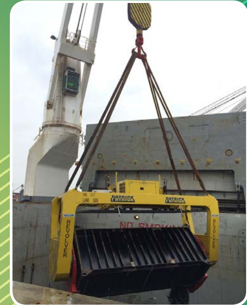
Containers being tipped into ships hull.
