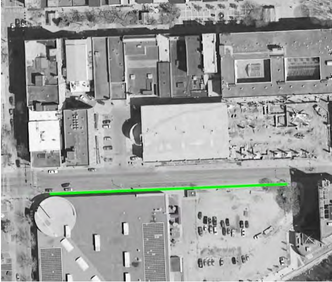
Location of the project. The green line represents a continuous trench of CU-Soil®
