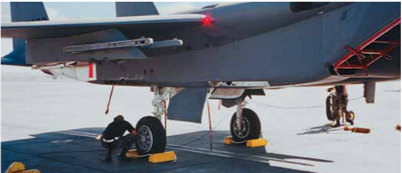
Checkers AC6820-LR aviation chocks used on a McDonnell Douglas F-15 Eagle
