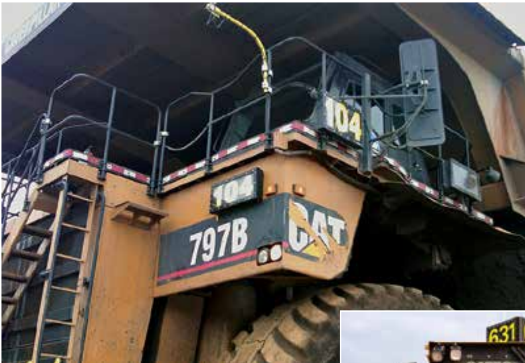
Rectangular Vehicle Identification Lights on the front of a 400-ton mine haul truck.
