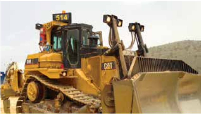
Triangular Vehicle Identification Light on a dozer.
