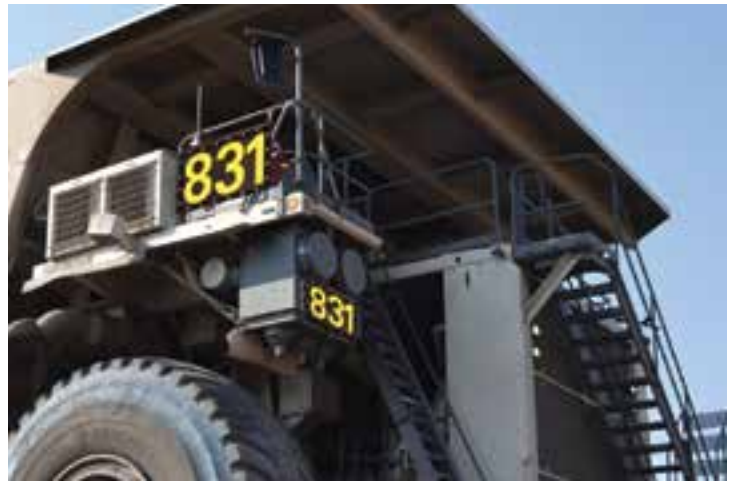
Rectangular Vehicle Identification Light on a 400-ton mine haul truck.
