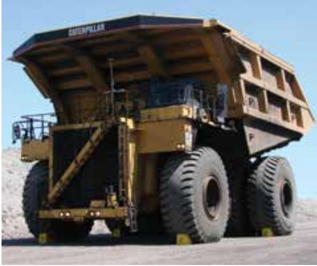
Four Checkers wheel chocks, model MC3011 used on CAT 797
