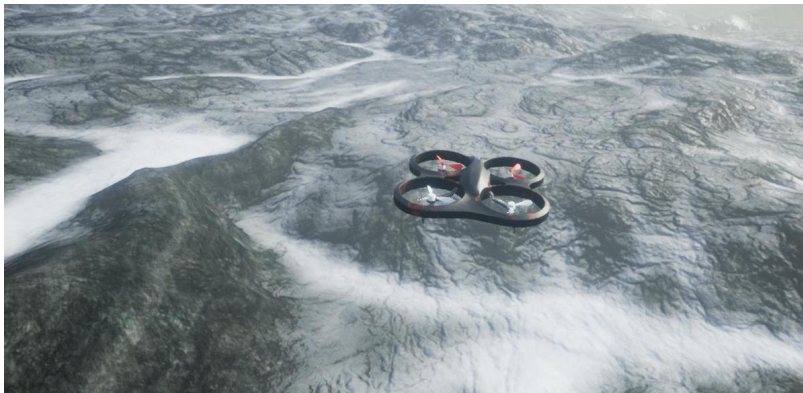
Figure 1: Quadrotor in AirSim Mountains Environment. We consider the problem of generating adversarial disturbances (e.g., wind gusts) for a given controller.
