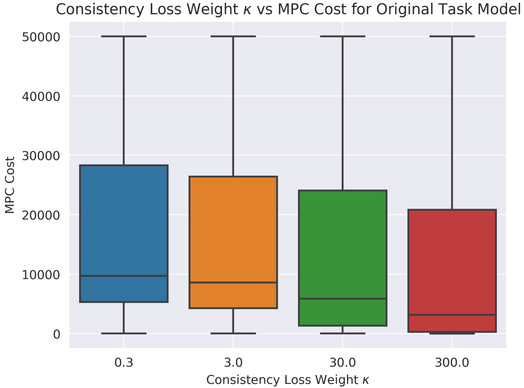
Figure 14: Consistency Loss Weight Ablation Study for Toy 2D Planning: The figure shows the relation of \kappa values to the MPC Cost of the corresponding synthesized adversarial scenarios for the Toy 2-D Planning experiment. On the x-axis, we have the \kappa value used in the adversary loss, Eq. 1, and on the y-axis, we have the corresponding MPC Cost. The plot shows that the user can easily control how adversarial the synthesized scenarios are by tuning the \kappa value. This plot also demonstrates that our loss function works as desired, as we can see the scenarios with higher \kappa values have lower MPC costs than scenarios with lower \kappa values.
