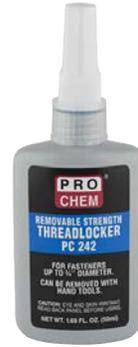
THREADLOCKER PC 242 is a medium strength, general purpose fastener adhesive. Cures only after adhesive is confined between mating surfaces. Will withstand temperatures of up to 300°F and most solvents. Eliminates the need for stocking lock washers, plastic inserts and locks, machine access bolts and hydraulic system bolts. Locks and seals while preventing parts from loosening due to vibration. Temperature range -60°F to +300°F. Fixture speed 15-20 minutes. Full cure 24 hours.
