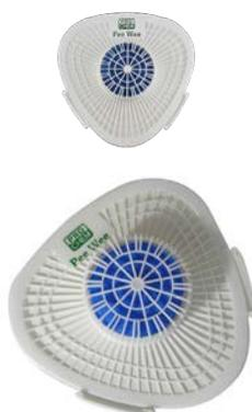
PEE WEE is a urinal screen designed to prevent drains from clogging and to keep urinals clean and smelling fresh. Each block contains over 3 billion enzyme-producing biocultures that destroy organic materials that cause odors. The urinal screens feature a raised holder to keep deodorant block dry, lengthening block life. It is made from pliable plastic to fit the contour of any urinal, and offers break-off hooks for easy, sanitary replacement.
