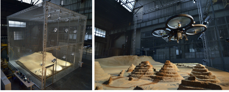
Fig. 2. Left: the Vision-based Navigation Facility. Right: the drone flying (note the camera facing down observing the diorama).
