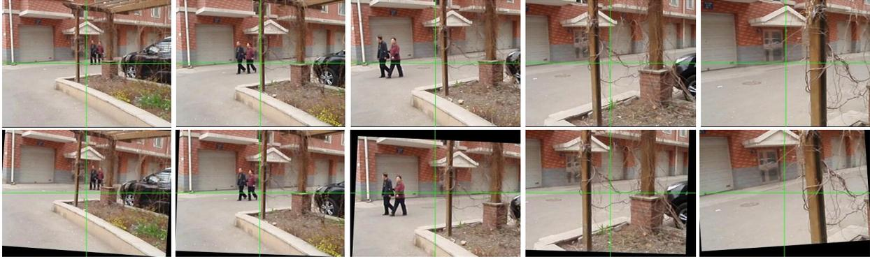
Figure 5: The results of the proposed video stabilization algorithm. Images in the first row are original frames, and images in the second row are the video stabilization results.
