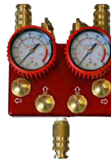
Dual Push Button Deadman control with 120 psi/8 bar relief valve used to control inflation and deflation with one common air source of Matjack high pressure air lifting bags, come standard with two 0-160 psi/10 bar gauges.
