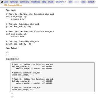
Fig. 7: View of progressively fillable notebook after user has completed Step 1. The last version of code entered and executed by the user is included the markup, and the code cell now displays the "correct" version of the code. Note the comment suffix ## ANSWER on selected lines of code. These lines were hidden in the unfilled view.
