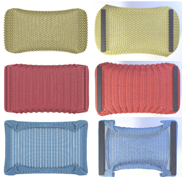
Fig. 11. Comparison of yarns animated with our method applied to a pre-computed cloth simulation (left) against full yarn-level simulation (right, courtesy of Sperl et al. [2020]). Our yarn level deformations differ the most where the triangle-level cloth simulation is least accurate.
