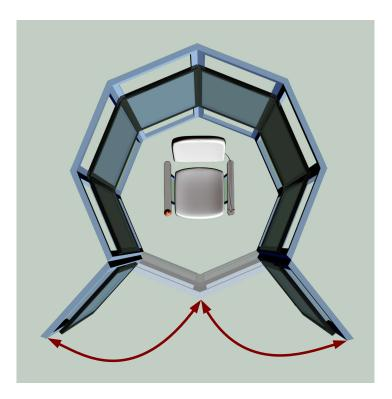
Figure 3.3: The OctaVis viewed from the top. Two displays act as door segments and allow to easily enter the system.
