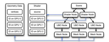
Figure 4.1: Scenegraph nodes share data through shared OpenGL contexts to reduce memory consumption.
