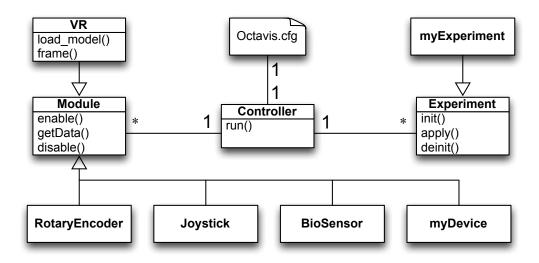
Figure 4.5: UML diagram of the main software architecture.
