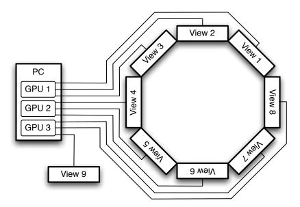
Figure 3.5: Schematic view of the rendering setup. One PC, equipped with three GPUs, drives the eight VR displays and an operator display.
