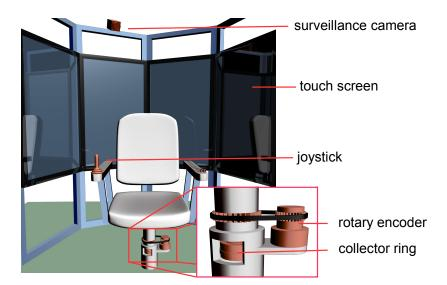
Figure 3.2: Illustration of the navigation and interaction components. The orientation of the chair, determining the movement direction, is measured by a rotary encoder and a "throttle joystick" in the armrest adjusts the speed of movement. Easy and natural interaction with objects is enabled through a simple touch screen interface.
