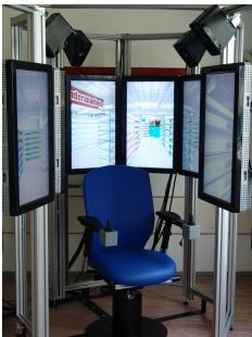
Figure 3.1: Two photographs of the OCTAVIS system. Eight screens, arranged in an octagon, provide a 360° panorama visualization of the virtual environment. Two door segments can be opened (right). Navigation in the VR is performed through a modified office chair, whose orientation determines the movement direction, and a "throttle joystick" in the armrest. Easy and natural interaction with objects is enabled through a simple touch screen interface.
