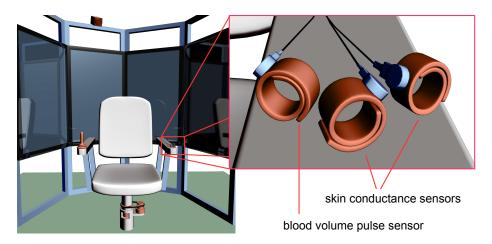
Figure 3.7: Illustration of the OCTAVIS system with a close-up of the skin conductance and blood volume pulse sensors used for patient monitoring.
