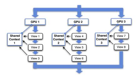
Figure 4.2: All views attached to the same GPU share a render context and are drawn consecutively, while the rendering is parallelized over the available GPUs.
